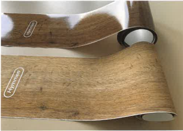
Fig. 6a: Digitally printed décor paper by Saturn before (bottom) and after impregnation (top)
