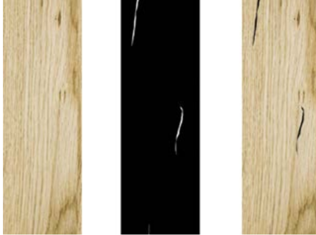
Adding characteristics, such as cracks, knots or colouring using a digital printing mask
