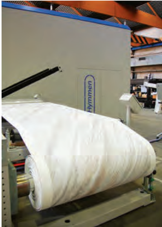
Picture 1: Hymmen JUPITER Digital Printing Line for printing on foils or paper
