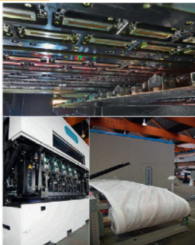
The Hymmen JUPITER Digital Printing Line: JPT-WS for edge-banding material and JPT-W for paper and foils
