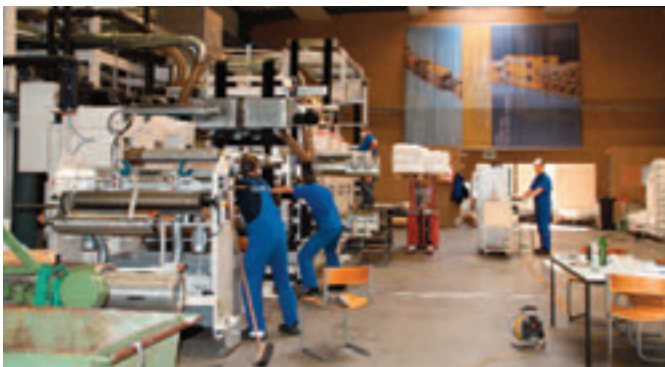
>The Rödinghausen pilot plant is equipped with examples of all the main machinery products from every part of the company. Customers can bring in their own materials for test production runs.
